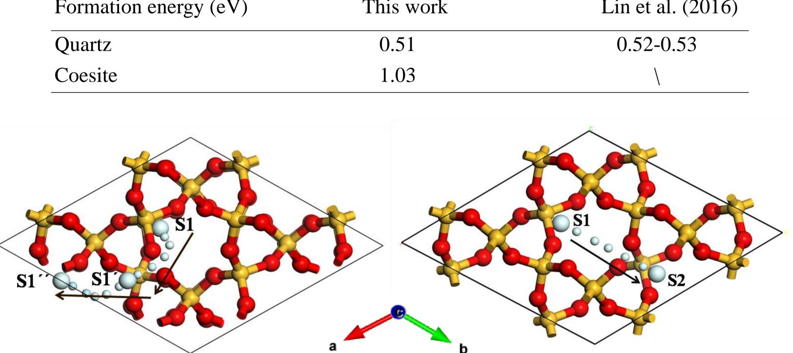
Fig. 1. Diffusion pathways of helium atom in quartz along [010] via the S1'site and reaching the S1''site and along [100] reaching the S2 site.
