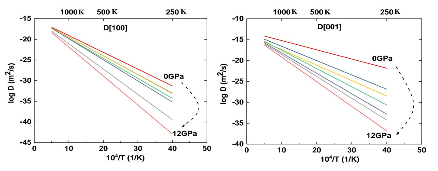
Fig. 5. Effect of pressure on helium diffusion in coesite up to 12 GPa in the [100] and [001] directions.
